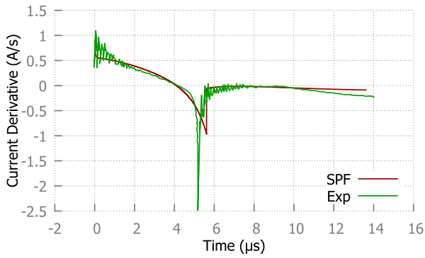
Fig. 3. Current derivatives corresponding to the discharge currents in Figure 2 for DT mixture.
