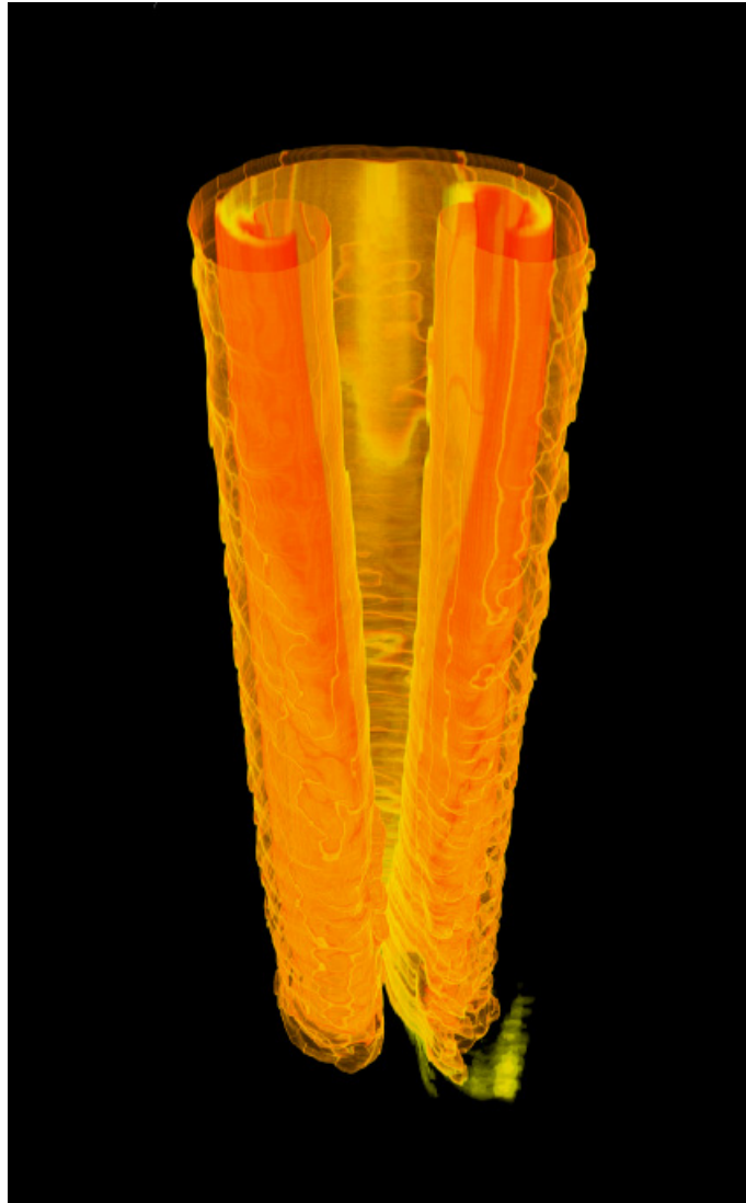
Figure 4: The flowfield density illustrates the vortex structure induced in a column of sulfur hexafluoride 825 \mu\text{s} after the passage of a Mach 1.2 shockwave. The shock induces vortical motions because of the misalignment between pressure and density gradients characteristic of the shockwave and the column material. Small-scale irregularities also develop because of fluid dynamic instabilities. The data is from a three-dimensional numerical simulation that was carried out using the FLASH code running on the ASCI Q machine. The initial conditions match experiments carried out at Los Alamos National Laboratory. FLASH is a parallel adaptive-mesh-refinement numerical hydrodynamics code developed at the ASCI Alliances Center for Thermonuclear Flashes at the University of Chicago. Visualization was produced using software developed in collaboration with Argonne National Laboratory.
