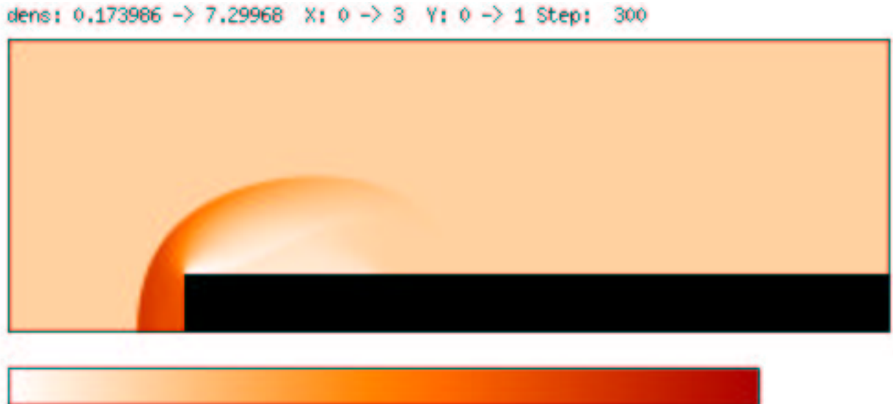
Figure 16.1: Density in the windtunnel setup, as rendered by the runtime visualization module
