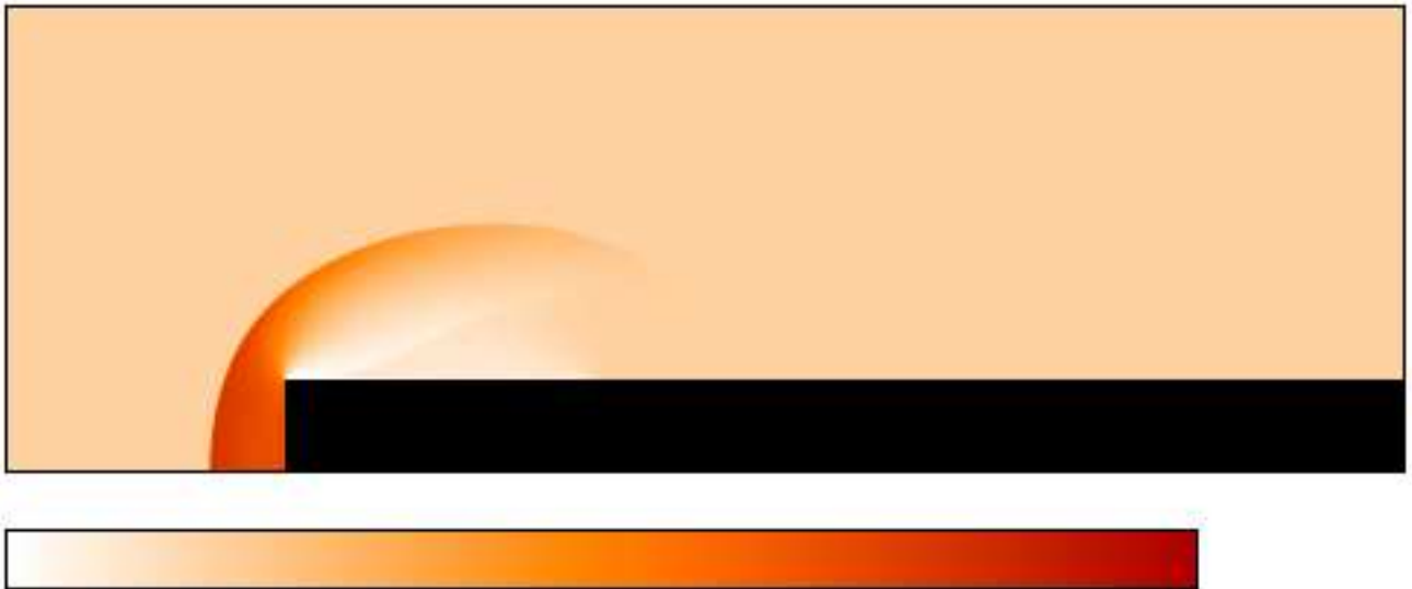
Figure 16.1: Density in the wind tunnel setup, as rendered by the runtime visualization module
