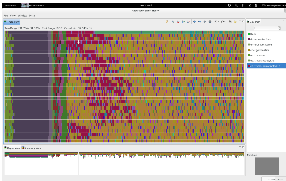
Figure 18.16: Performance trace of MPI ranks 0-33 in a laser simulation using asynchronous communication and run with 2048 MPI ranks on Intrepid BG/P.
